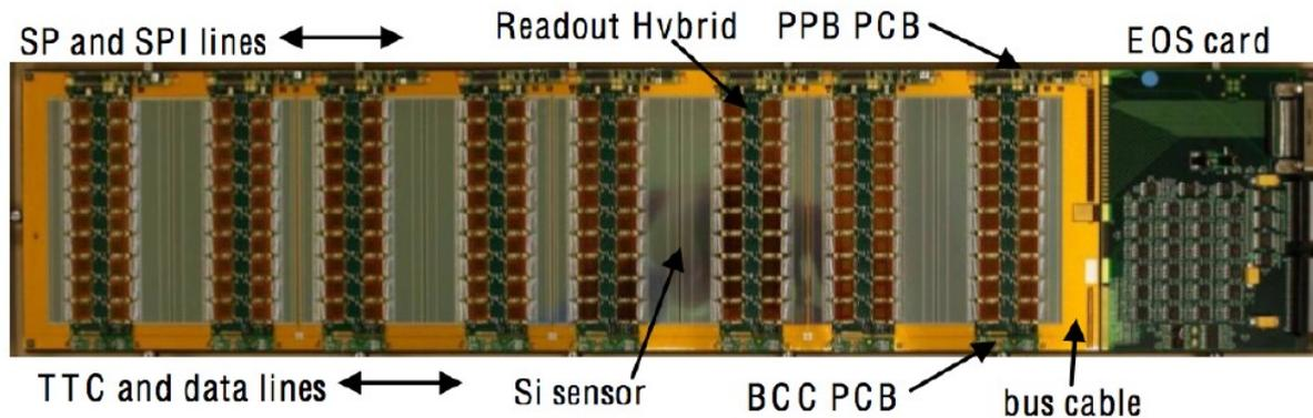
Figure 1. Photograph of the 4-module stavelet with ABCN-25 readout and all circuits required for serial powering.
