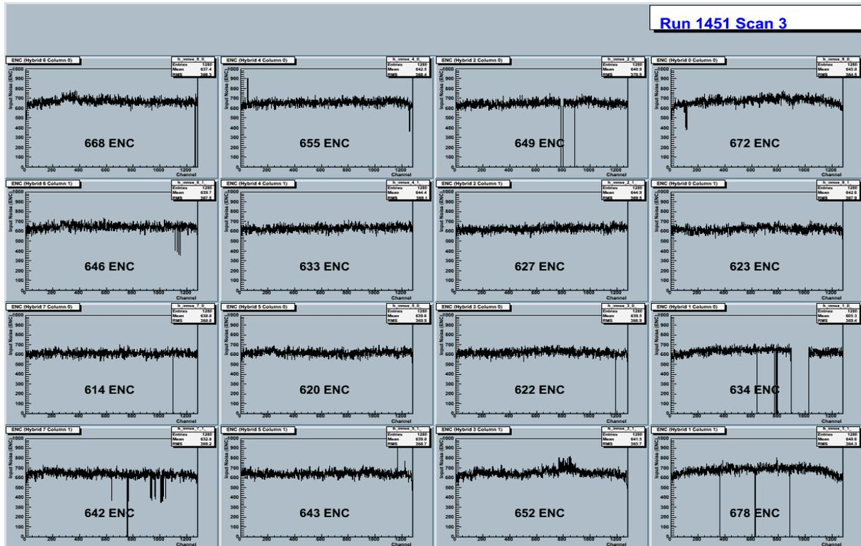
Figure 2. Noise measured for the entire stavelet powered serially. Each plots shows the Equivalent Noise Charge (ENC) across 1280 readout channels, i.e. 10 ABCD-25 chips, and the mean values of ENC.
