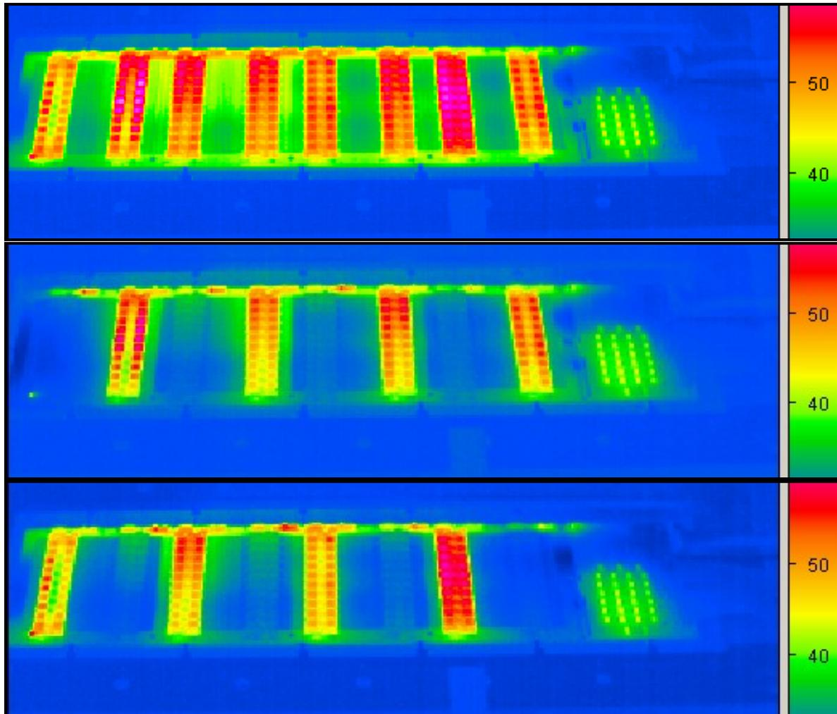
Figure 3. Infrared images of temperature distribution on the hybrid for all hybrids powered (upper), odd hybrids bypassed and even hybrids powered (middle) and odd hybrids powered and even hybrids bypassed (lower).
