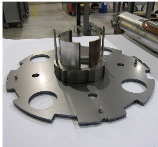
Figure 22: MCXB verification of assembly parameters on prototype parts (coil arches, collar packs and yoke laminations)
