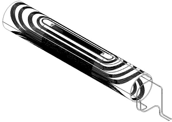
Figure 5: 3D view of the 855-mm-long MCXB coil
