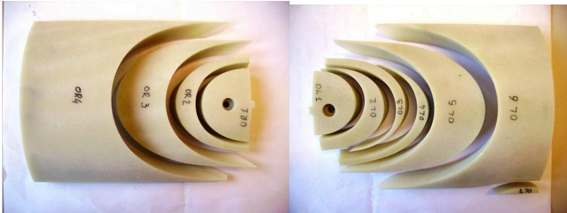
Figure 1: Production set of end-spacers for the outer layer coil of MQXC
