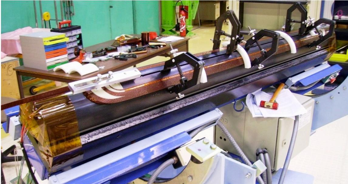
*Figure 3: Winding of the first production coil at CEA/Saclay.*
