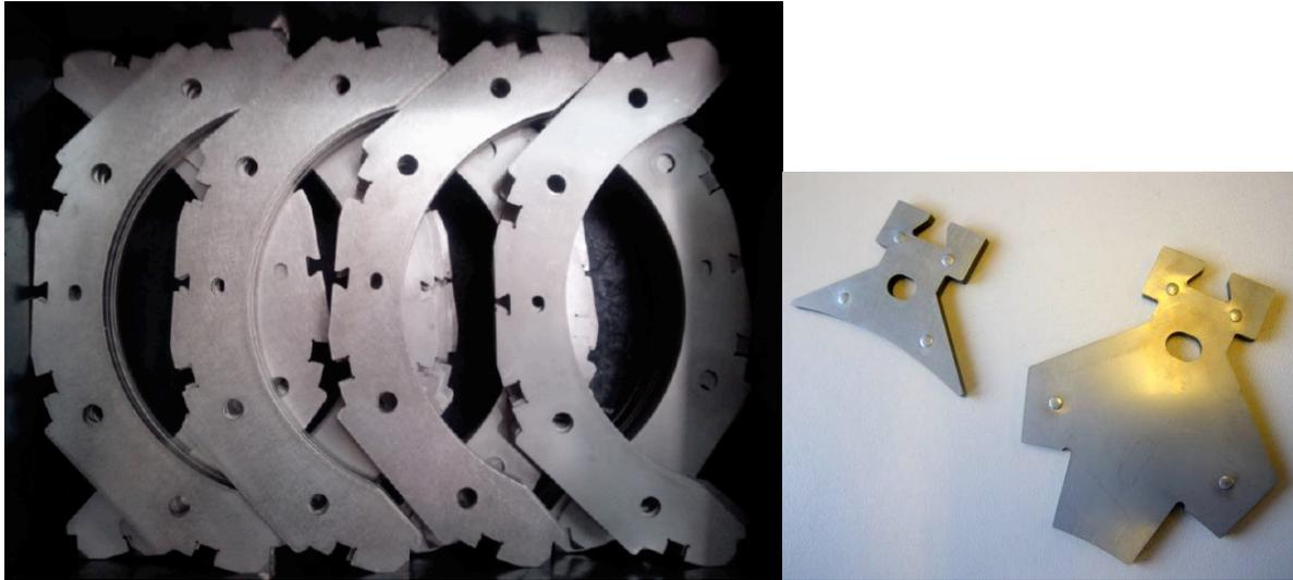
Figure 6: Left: Production batch of collar laminations for the end-section of the magnet (covering the coil ends with the G11 endpacers). Right: Insert collars with dimples.
