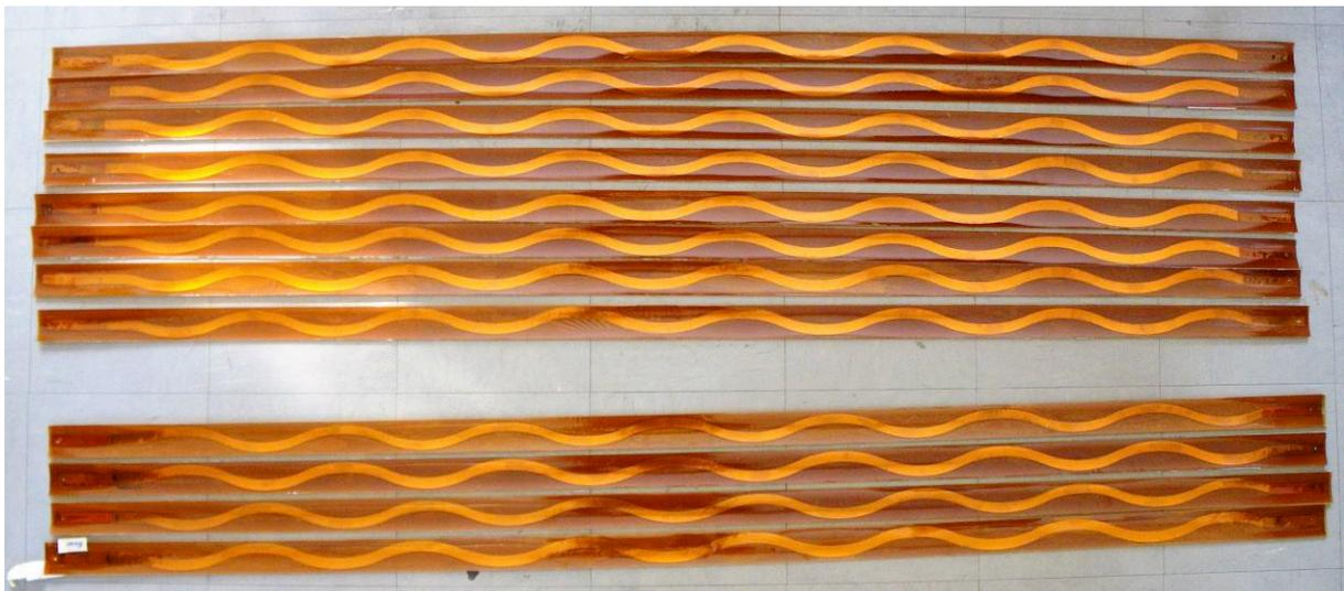
Figure 7: Production batch of quench heaters.
