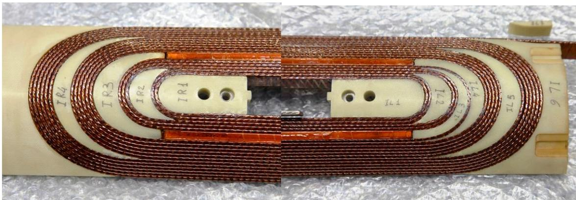
Figure 2: Extremities of the first (inner layer) production coil wound at CEA/Saclay. Left: Return end, Right: Lead end.
