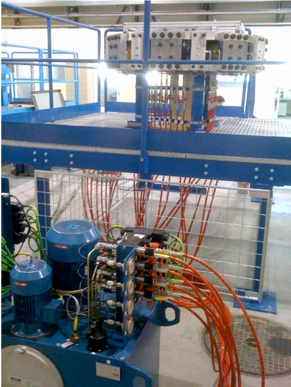
*Figure 12: Collaring press with hydraulic elements*
