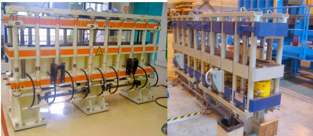
Figure 8: Left: Curing press for the 2-m-long superconducting coil at CEA/Saclay. Right: Curing press at CERN
