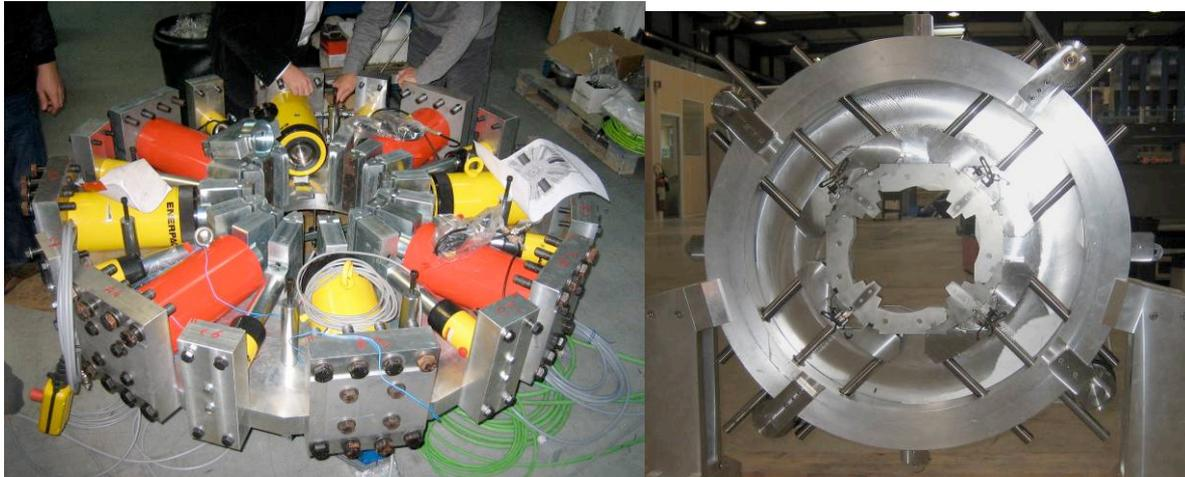
Figure 13: Left: View of the press anvils before the mounting of the cover flange. Right: Pre-assembly tooling with collar packs attached.
