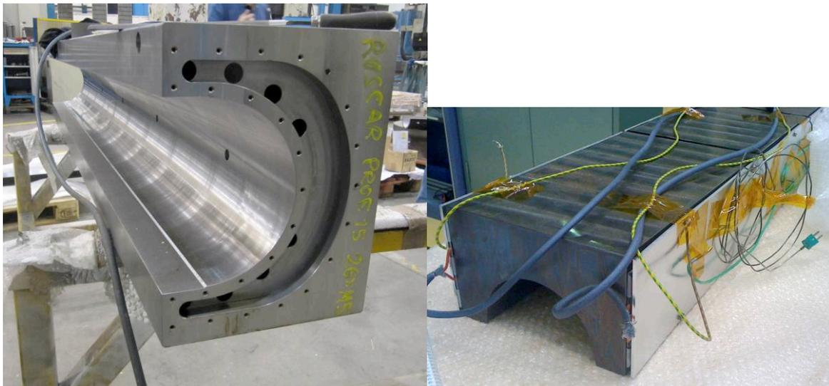
Figure 9: Left: Curing mould with channels for the oil heating. Right: Mould with heating plates
