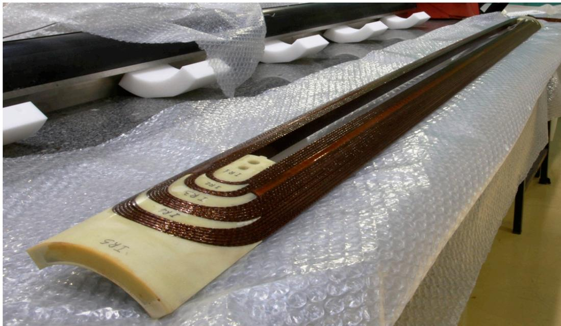
*Figure 4: Photograph of the first (inner layer) production coil for the MQXC quadrupole magnet produced at CEA/Saclay.*
