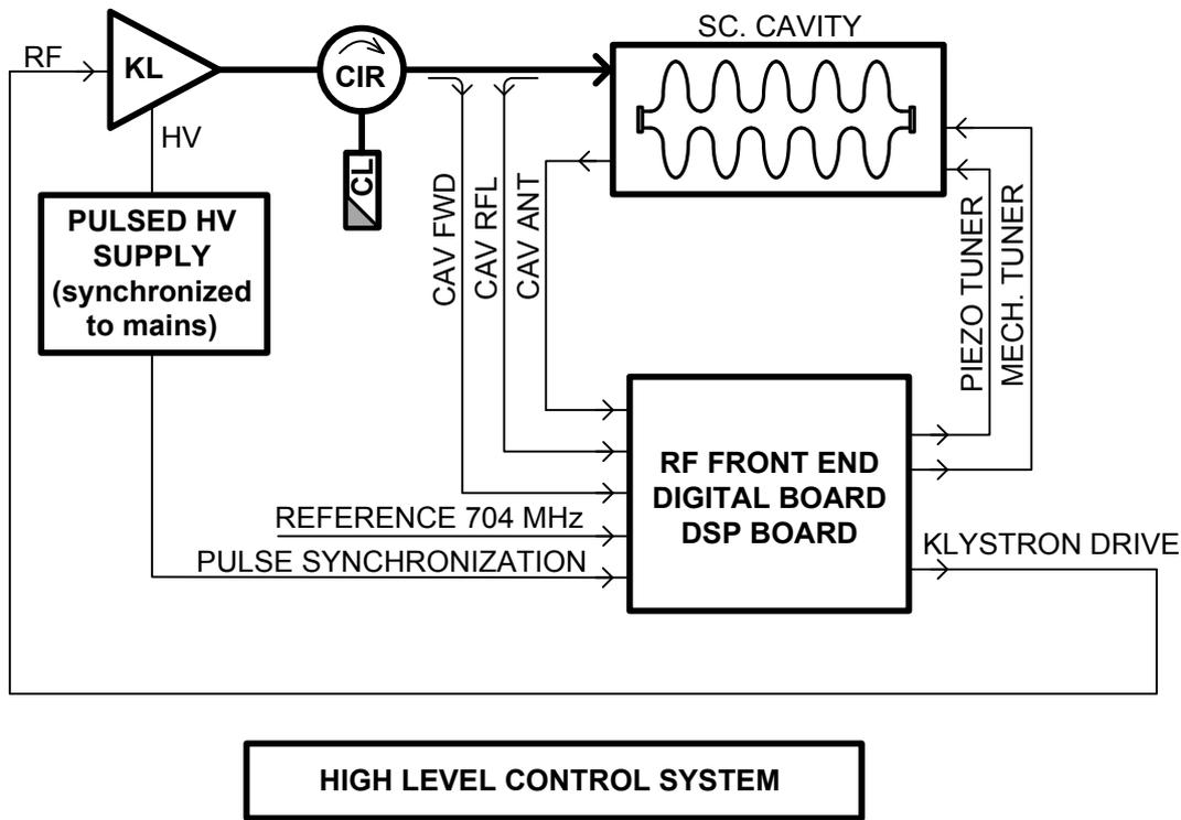
Fig. 4 Block diagram of the complete RF test installation
