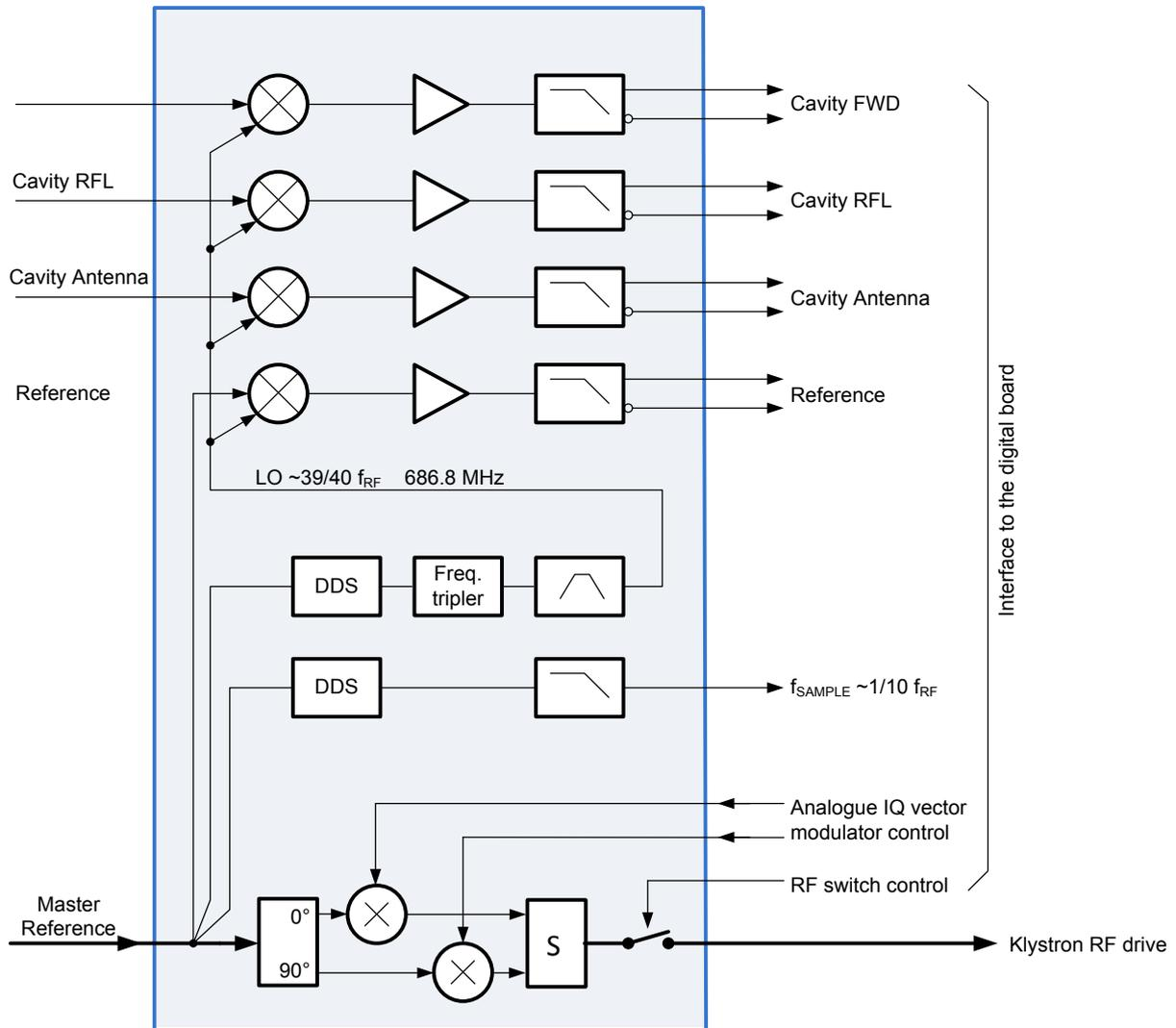
Fig. 5: Block diagram of the RF front-end module
