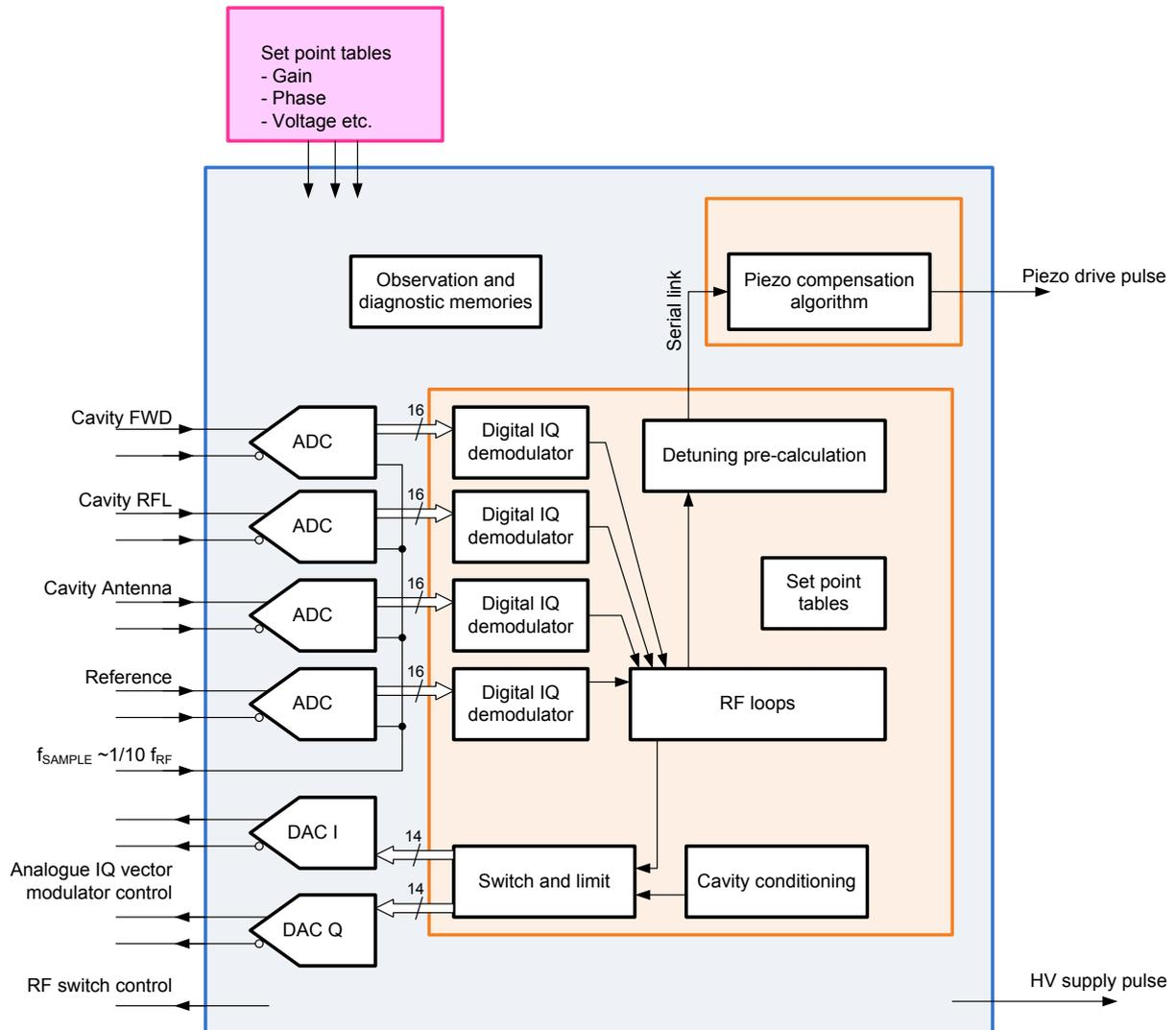
Fig. 6: Block diagram of the digital board
