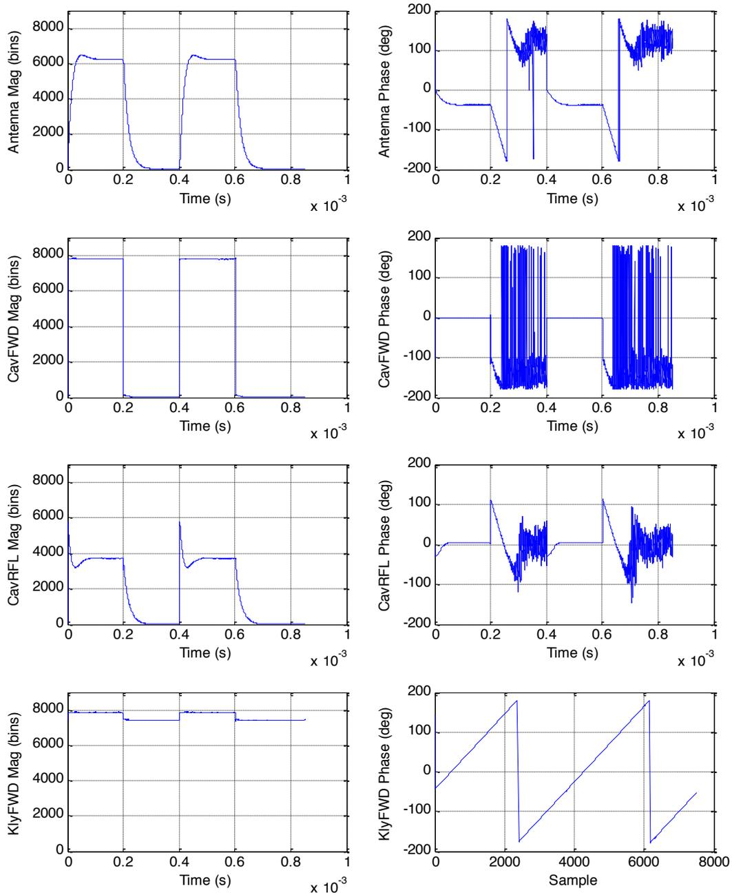
Figure 3: Cavity filling transient, cavity detuned by a fraction of a bandwidth, calibrated and corrected data
