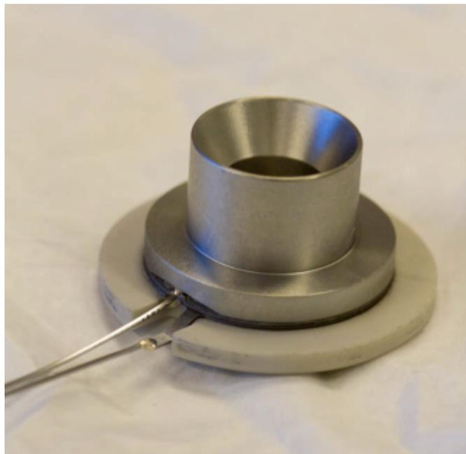
**Figure 24:** Brazed electrode assembly consisting of the funnel and aperture electrodes, the separating AlN insulators, and the electrical connections.
