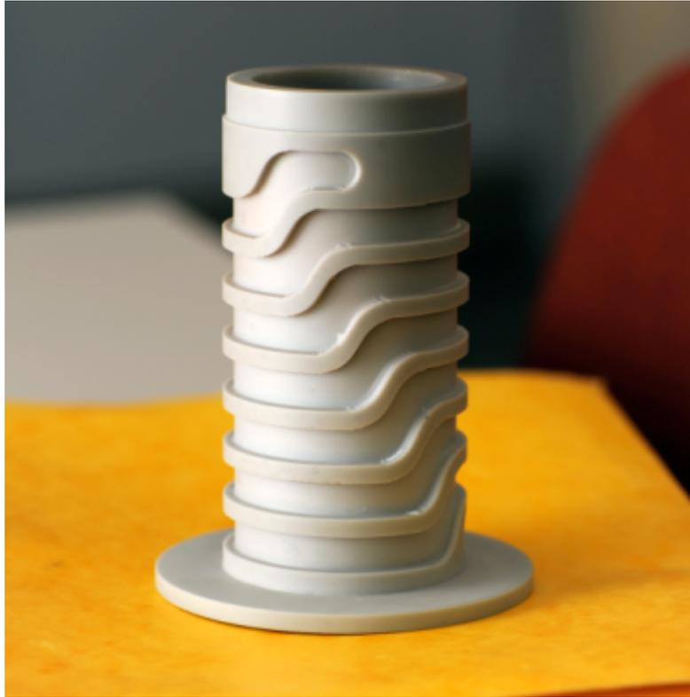
*Figure 10:* Installed AlN ceramic plasma chamber.
