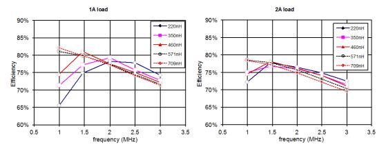
Figure 1: efficiency of the AMIS2 ASIC at 1A and 2A output currents.
