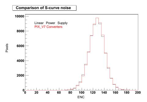
Figure 15: Measured noise distribution (width of the S-curve) for a current pixel module when powered with a linear lab power supply (black) or with two PIX\_V7 DC-DC converters.
