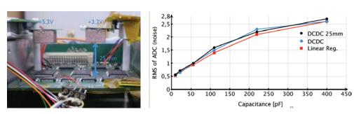
Figure 13: noise performance of the CMS HCAL front-end system using a linear power supply and the SM01C converters.
