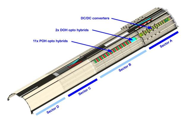
Figure 14: the supply tube of the CMS pixel detector as planned for the Phase-1 Upgrade. DC-DC converters will be integrated at the far end, in sector A, at a distance of about 2m from the pixel modules.
