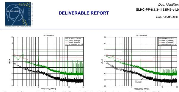
Figure 4: Common Mode (left) and Differential Mode (right) emissions of the AMIS2\_EMC prototype (in black) compared to those of Proto5 (in green).
