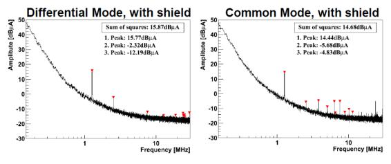
Figure 7: Differential and Common Mode noise spectra measured at the output of the PIX\_V7 DC-DC converter for an input voltage of 10V, an output voltage of 3.3V and a switching frequency of 1.3MHz.
