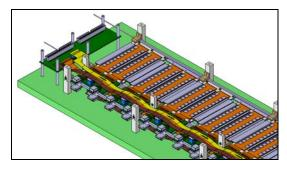
Figure 12: supermodule implementation of the ATLAS tracker using the SM01C converters.
