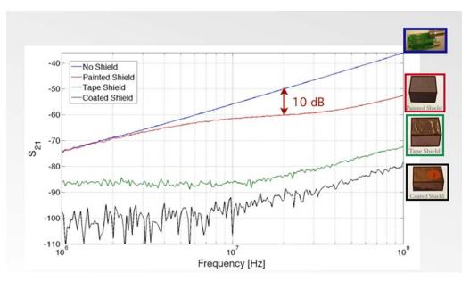
Figure 5: shielding effectiveness of copper painted shields, copper taped shields and copper coated shields
