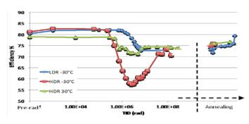
Figure 2: efficiency of the AMIS2 ASIC as function of the total ionizing dose.
