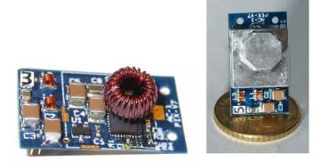
Figure 6: The PIX\_V7 DC-DC converter developed at the RWTH Aachen university.
