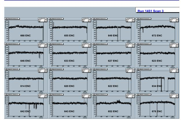
Figure 2. Noise measured for the entire stavelet powered serially. Each plots shows the Equivalent Noise Charge (ENC) across 1280 readout channels, i.e. 10 ABCD-25 chips, and the mean values of ENC.
