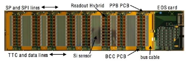
Figure 1. Photograph of the 4-module stavelet with ABCN-25 readout and all circuits required for serial powering.
