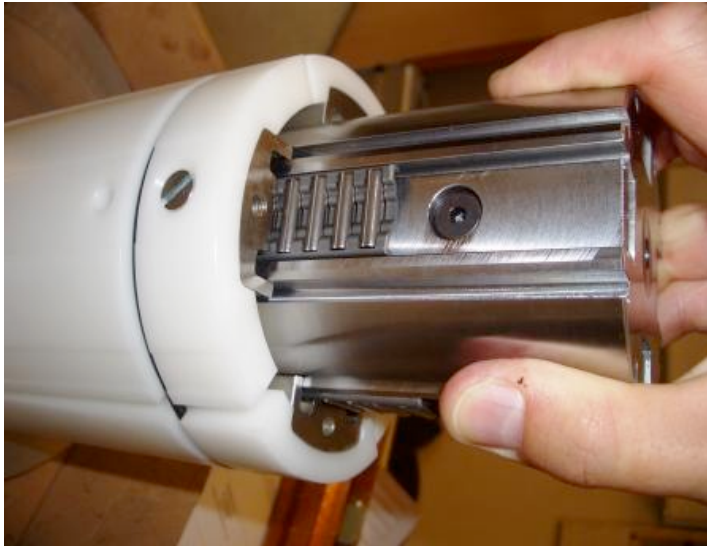
Figure 3: Split mandrel procured from European Industry
