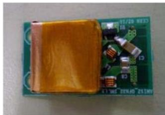
Figure 3: AMIS2\_EMC prototype converter with shield.
