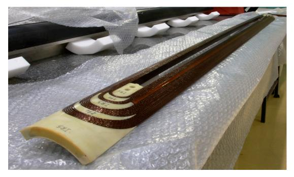
Figure 4: Photograph of the first (inner layer) production coil for the MQXC quadrupole magnet produced at CEA/Saclay.
