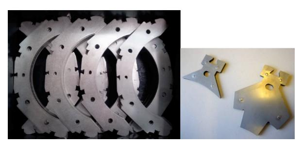
Figure 6: Left: Production batch of collar laminations for the end-section of the magnet (covering the coil ends with the G11 endpacers). Right: Insert collars with dimples.
