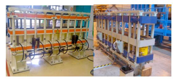
Figure 8: Left: Curing press for the 2-m-long superconducting coil at CEA/Saclay. Right: Curing press at CERN
