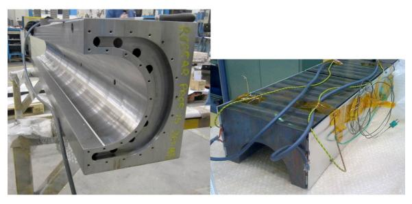
Figure 9: Left: Curing mould with channels for the oil heating. Right: Mould with heating plates
