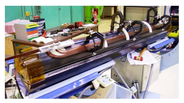
Figure 3: Winding of the first production coil at CEA/Saclay.
