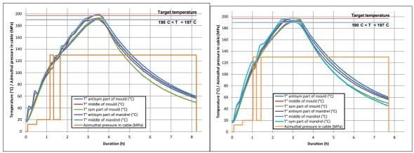
*Fig. 10: Measurement of the coil temperature during the curing of inner layer coil (left) and outer layer coil (right)*
