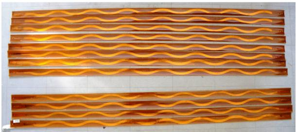
Figure 7: Production batch of quench heaters.
