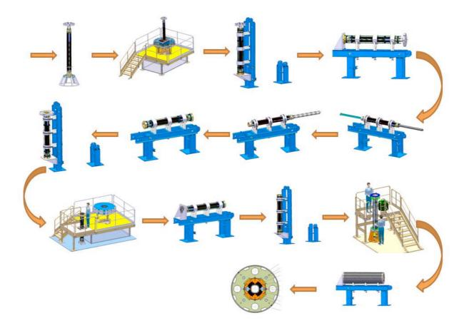
Figure 11: Assembly sequence of the MQXC quadrupole magnet
