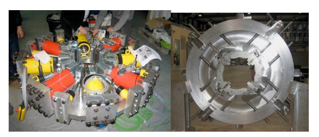
*Figure 13: Left: View of the press anvils before the mounting of the cover flange. Right: Pre-assembly tooling with collar packs attached.*
