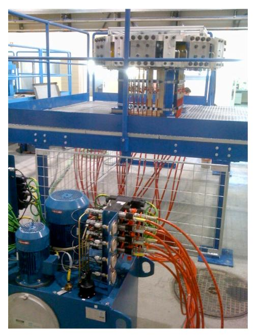
Figure 12: Collaring press with hydraulic elements
