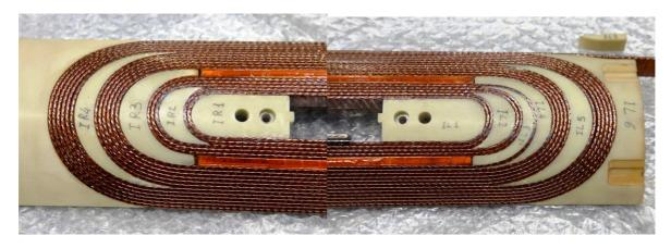
*Figure 2: Extremities of the first (inner layer) production coil wound at CEA/Saclay. Left: Return end, Right: Lead end.*
