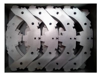
Figure 5: Production batch of collars for the central section of the magnet
