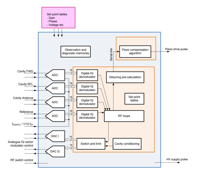
Fig. 6: Block diagram of the digital board
