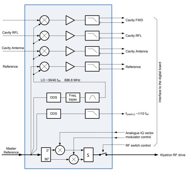
Fig. 5: Block diagram of the RF front-end module
