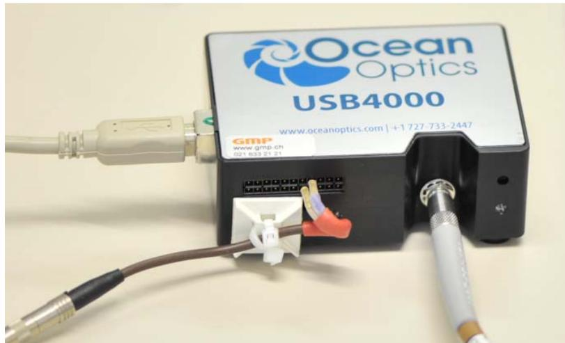
**Figure 53:** Trigger able fast spectrometer Ocean Optics USB4000 featuring a minimal light collection time of 4 ms and a dynamic range of typically 60. Also visible are the USB cable, the light fiber and the trigger cable.
