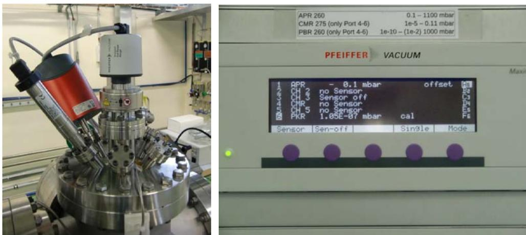
**Figure 31:** Left: top flange equipped with APR 260 (steel), CMR 375 (red) and PKR 261 (grey) pressure gauges. Right: MaxiGauge pressure gauge control unit.
