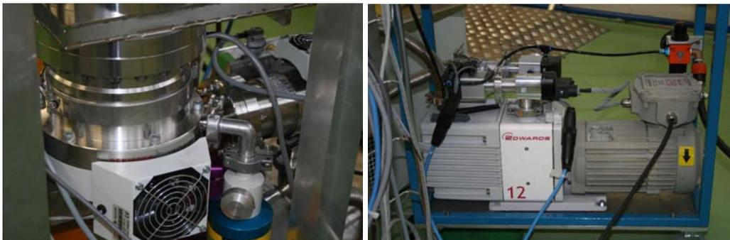
**Figure 74:** Left: TMU521 turbo molecular pump backed with a TMU071 turbo molecular pump.. Right: Edwards 12 roughing pump.
