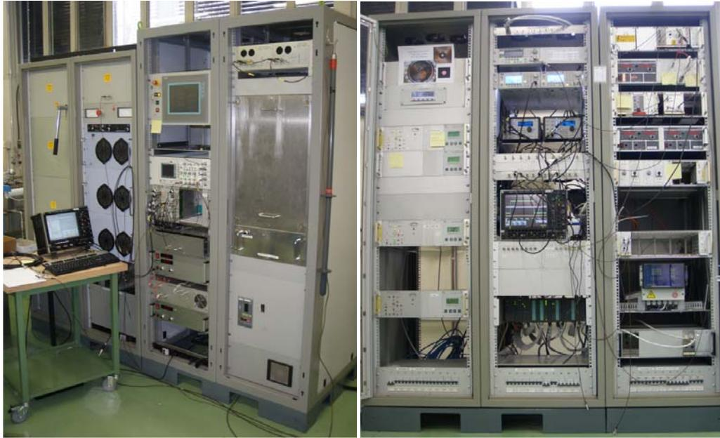
**Figure 24:** Left: High voltage and 2MHz RF generator. Right: Vacuum and controls racks.
