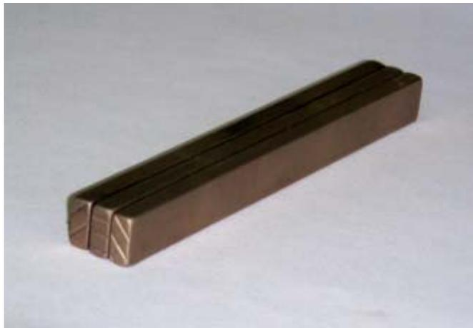
**Figure 16:** Photograph of an offset Halbach element.
