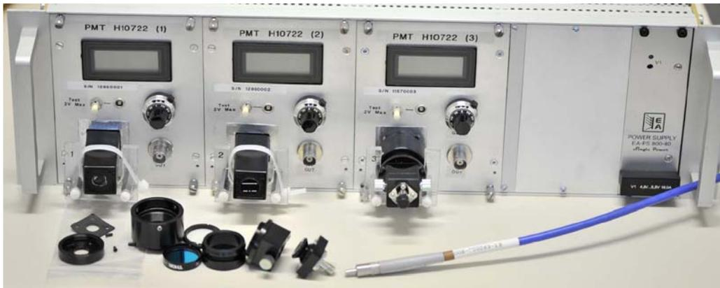
**Figure 56:** Real time measurement of up to three Hydrogen lines will be achieved with the Hamamatsu phototubes light detection system. The optical fiber is connected through a filter (10 to 40 nm FWHM) and attenuation box. The amplifier gain is tuned individually with a 10 turn potentiometer; its driving voltage is indicated at the mV level.
