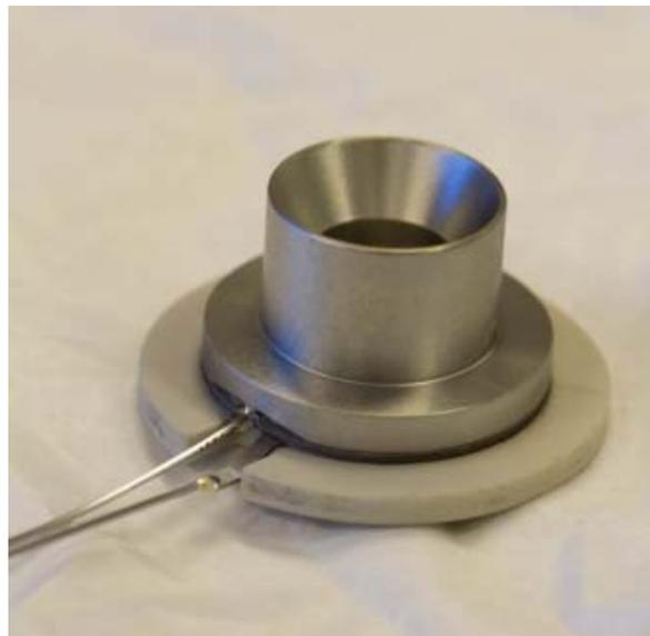
**Figure 19:** Brazed electrode assembly consisting of the funnel and aperture electrodes, the separating aluminum nitride insulators, and the electrical connections.
