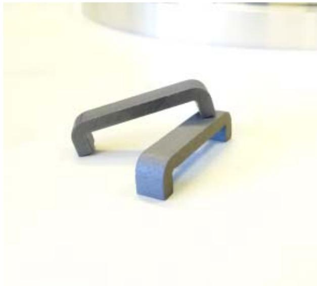
**Figure 15:** Two of the ferrites used in the SPL plasma generator.
