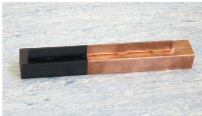
**Figure 41:** Cusp magnet with Cu housing used in the RF heating tests.
