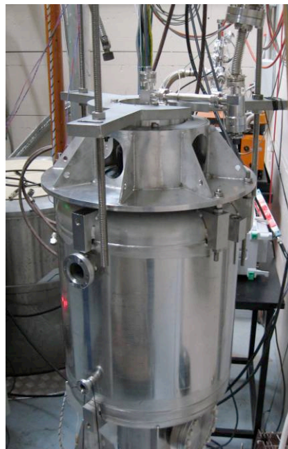
Figure 2.5: cavity setup with He tank and stiffener for vertical cryostat measurements.
