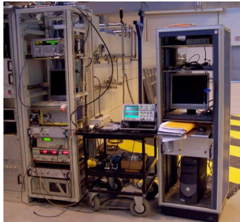
Figure 2.18: transfer function measurement and piezo control system (left rack) and stepper control system (right rack) sitting next to the Cryholab shielding.
