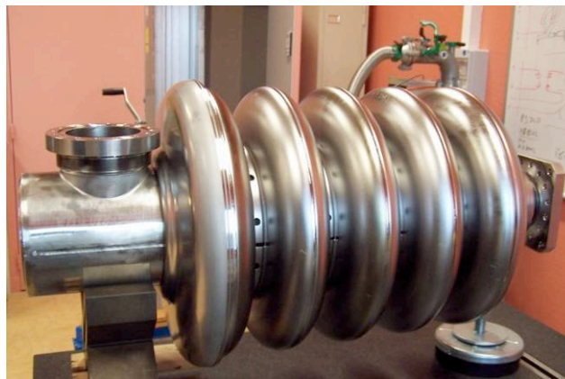
Figure 2.1: The bare Saclay 5-cell 700 MHz elliptical cavity.
