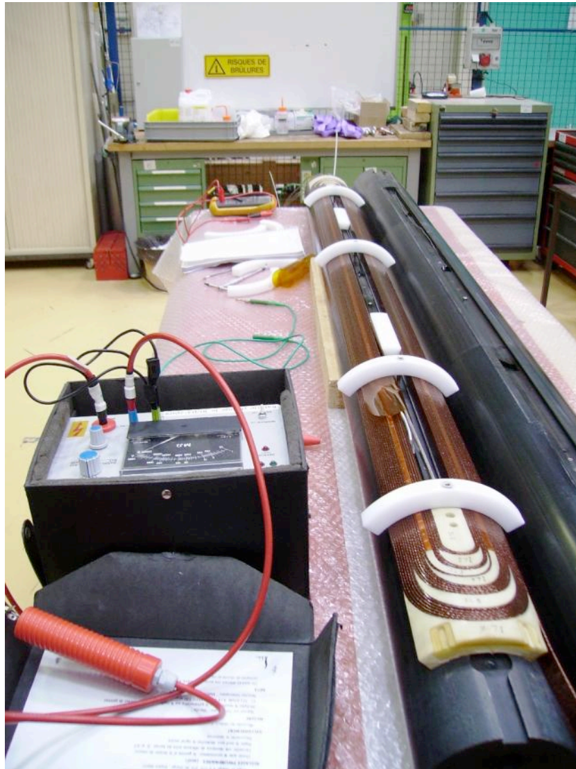
Fig. 2: Inner layer positioned on its mandrel connected to ground
