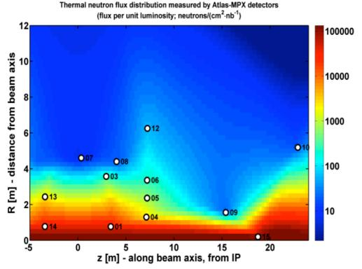
Fig.1): Measured spatial distribution (in one quadrant of the ATLAS detector) of thermal neutron fluence per unit luminosity. The iso-fluence curves are interpolated from measurements with the ATLAS-MPX network.
