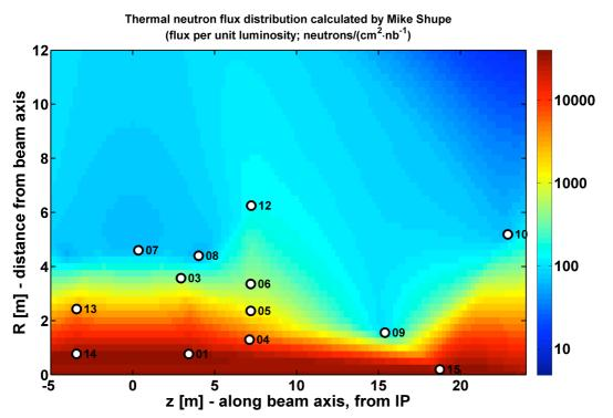
Fig 2): Predicted thermal neutron fluence per unit luminosity as calculated by PHOJET G3/GCALOR Monte Carlo simulations. The circles represent positions of individual ATLAS-MPX detectors (4 detectors are not shown in the figure).
