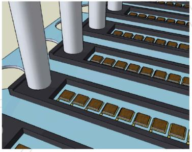
Figure 4.24: EDU detail showing linear arrays of SiPMs
