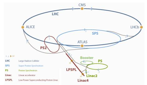
Figure 1: LHC and its injectors. During the SLHC-PP, Linac4 has been in construction for replacing Linac2, and the replacement of PS and PSB by LP-SPL and PS2 has been studied.
