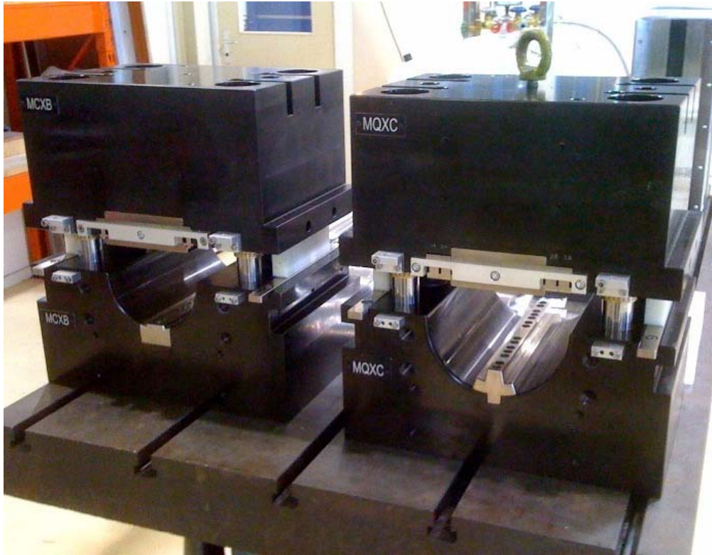
Fig. 9: Press inserts for measuring the coil size under the required azimuthal pressure.
