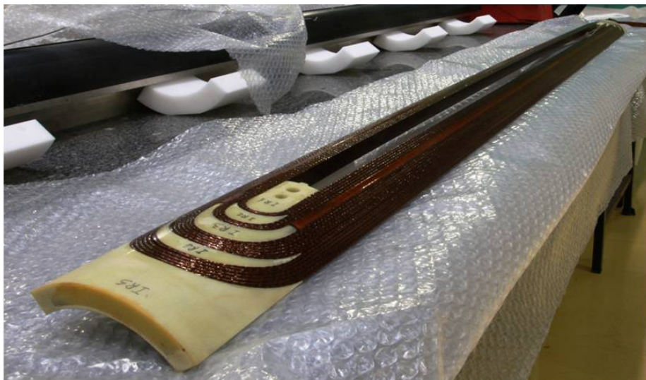
The four 'racetrack' coils form something of a gutter to allow the beam through. The ivory-coloured 'end spacers' neatly guide the cable in a smooth curve, keeping the magnetic field even all the way along the magnet.
