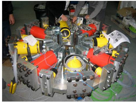
On the left, the hydraulics that provide the force in the collaring press, which tightens the collars and locks them in place. On the right, the assembled collar packs and mandrels inside the collaring press. The twelve anvils have evenly tightened the collars, and the box-shaped keys are inserted into the square chinks.
