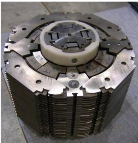
The plastic and metal 'assembly mandrel' protrudes from the centre of the stack of collars, with metal standing in for the coils. Its spring-loaded design makes it easy to disassemble and pull out of the collared coils.
